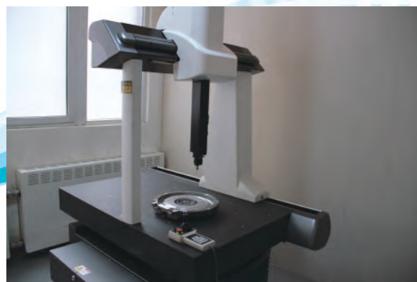
瑞典海克斯康三坐标 SWEDEN HEXACON THREE COORDINATE MACHINE
